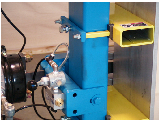
Lever Valve Locks Air Pressure For Glue Up Time
