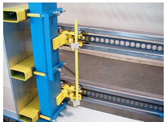
Drawbar Roller Carriage For Quick, Easy Changeovers
