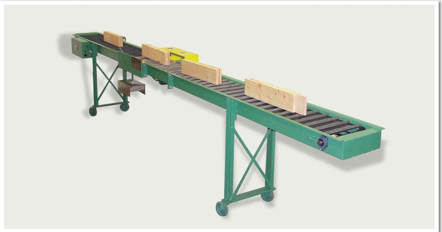
16' Conveyorized Glue Applicator with PVA Glue Pump
