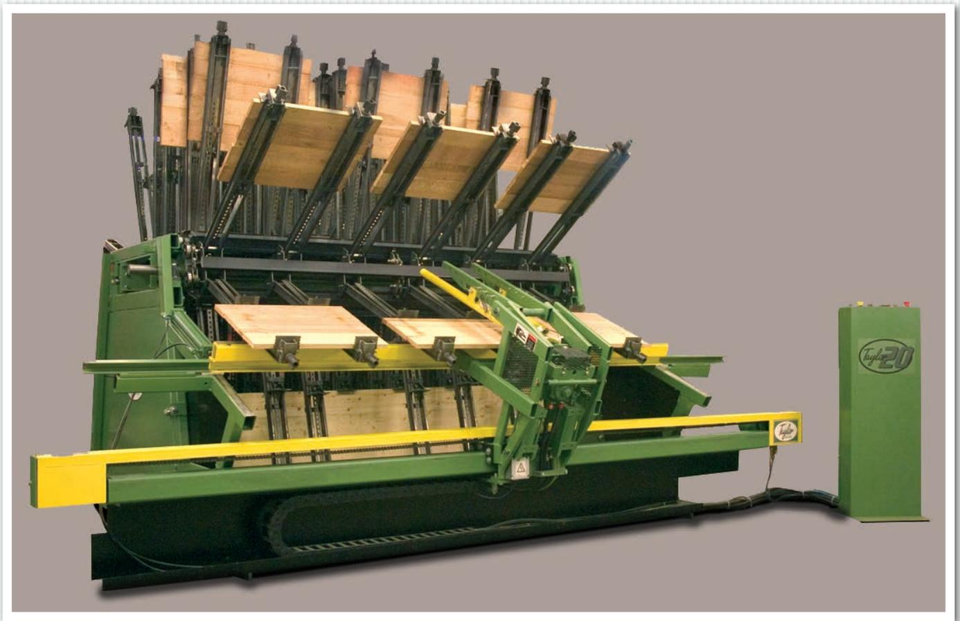
As stated earlier, the Automated Clamp Carrier also comes in a pneumatic version. The operation of the machine is identical to the hydraulic version, however, there are features to this machine that may be advantageous to your business:
