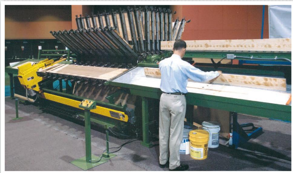
Side Loading Automated Clamp Carrier with Infeed Table and Glue Applicator, (mounted above infeed).
