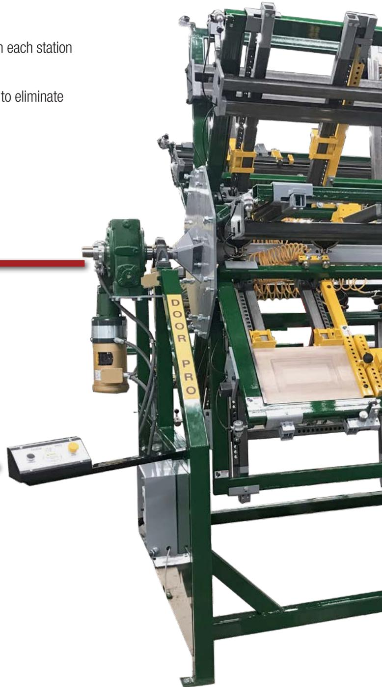
In a typical door shop glue is applied and components assembled on an assembly table. The door is placed in a section and clamps adjusted. The cylinders are activated by one valve which first creates side pressure pushing the door on the left side square, a second later the vertical clamps are activated to create pressure on the glue joints.
