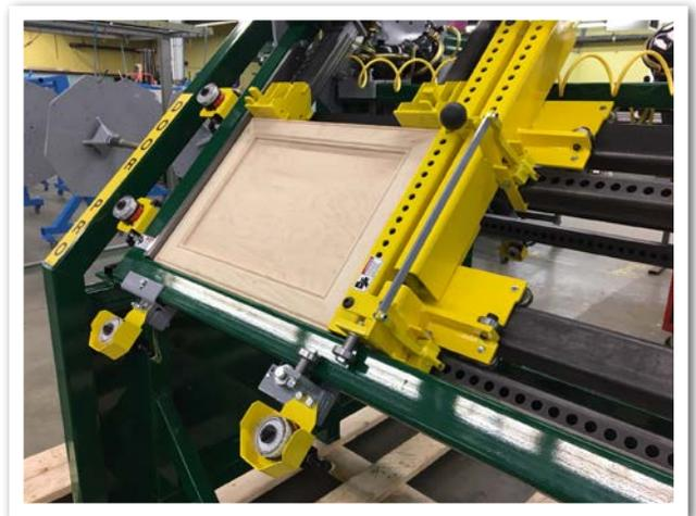
Clamp Doors Face Up to Eliminate the pinning process.
