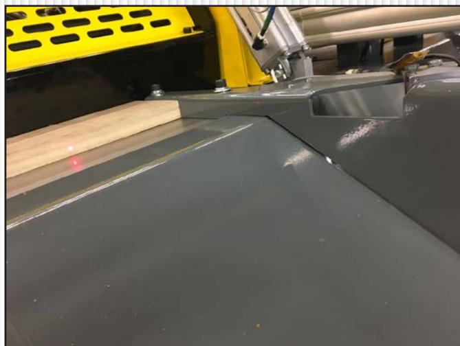
Board Width Sensor reading board
